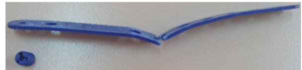
Fig. 5. Damaged fixing clamp
